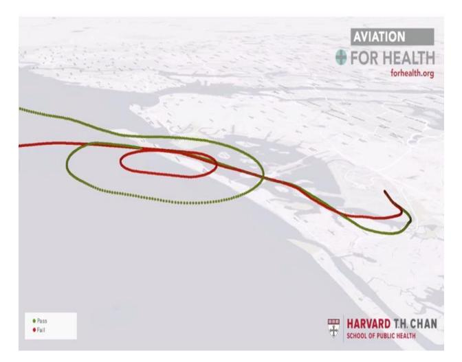
This study, published by Harvard professors in 2018<sup>11</sup>, was performed on experienced pilots using flight simulator trainers. The green (safe) flying pattern was flown when CO2 inside the cockpit was at 750 PPM. When the scientists manipulated the air quality in a way that raised the CO2 levels in the simulator up to 2,500 PPM CO2, the pilot's error rate, shown in red, soared.
