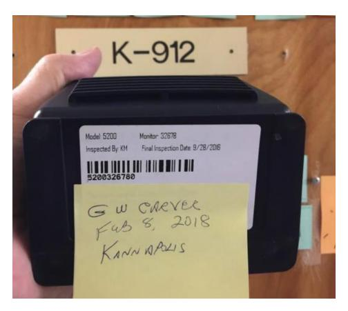
Each monitor, regardless of manufacturer, has a small fan, and an area where air is sucked in, and after electronic sampling, pushed out. This goes on continuously. It is vital that there be no external blockage of either intake or exhaust.
