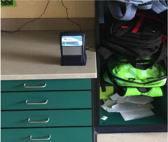
Here are two examples of bad placement. In the first, you can see that the back vent, where air is supposed to exit the monitor, is blocked. In the second photo, the monitor is placed on top of some device that is likely to influence monitor readings.
